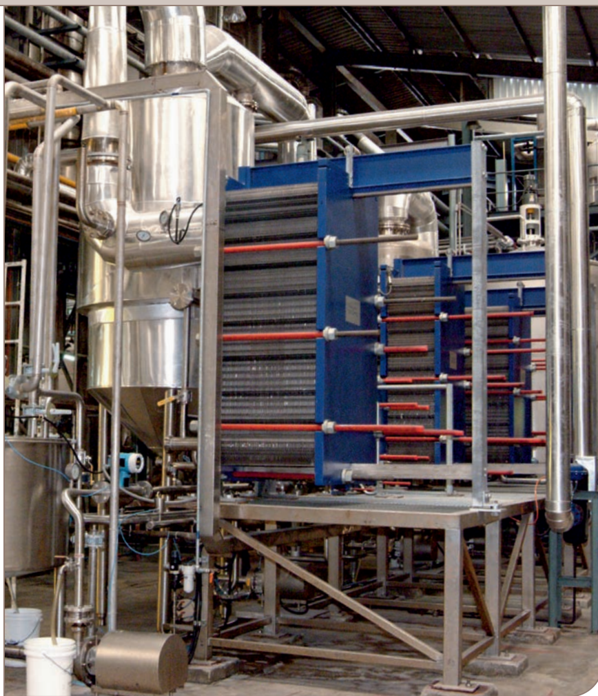
Three-effect AlfaVap plate evaporator system for fructose installed at Thai Glucose Co. Bangkok.
