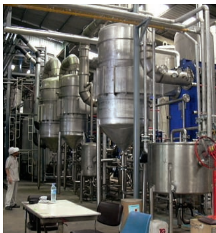
Two-effect AlfaVap plate evaporator system for dextrose and maltose.
